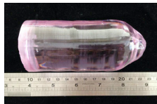
Above: YAG laser crystal, Taiwan Applied Crystal Ltd.
